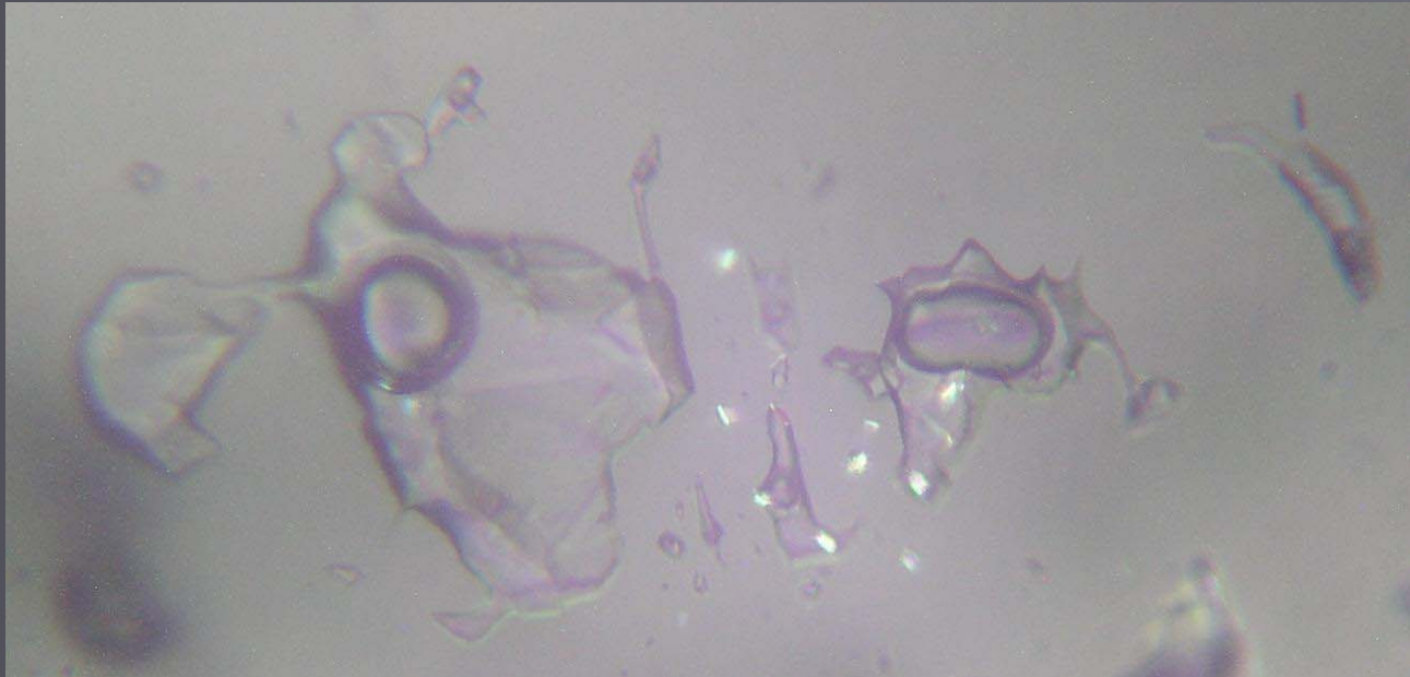
Secondary(?) gas-liquid FI with anisotropic satellite minerals
