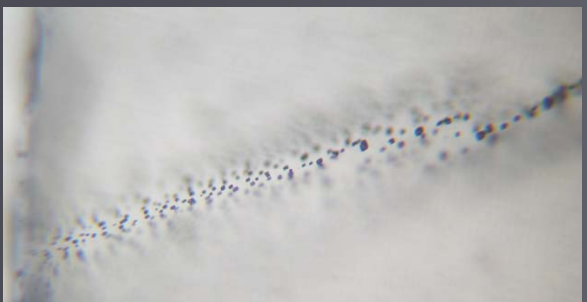
Secondary (?) FI in sub vertical fracture
